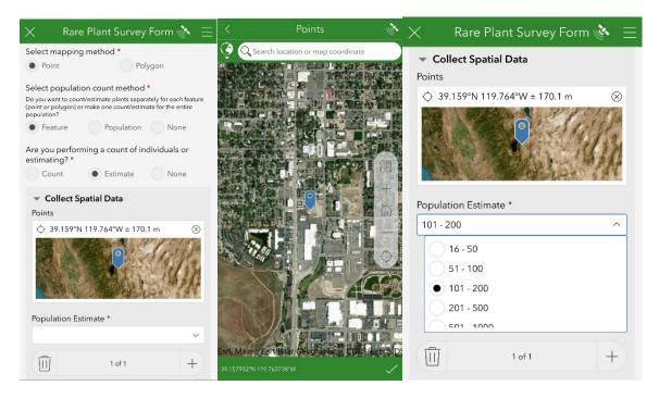
Simply clicking the plus sign will automatically collect a point. The form will display coordinates (WGS 84, decimal degrees) and precision (+/- X meters).
