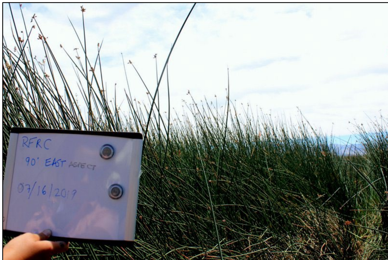
Figure 6. Example AA photo placard. Note placement of photo placard in corner and information written on placard: Point code, Aspect, and Date.
