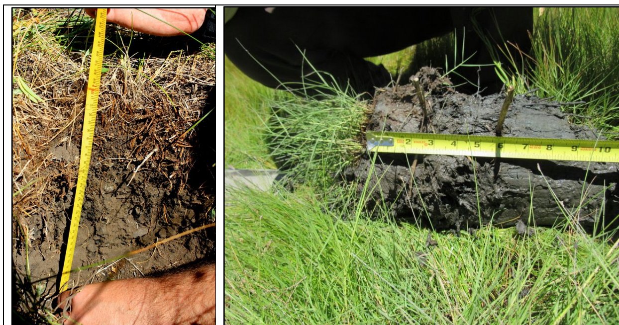
Figure 8. Soil Profile Description procedures pictured here: (at left) determining soil pit depth with a measuring tape, and (at right) removing a soil core in order to identify and mark the soil horizon depths using small sticks at 3 cm and 6 cm.
