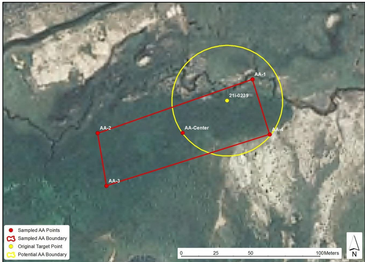
Figure 4. Map of rectangular AA adjusted from the target AA-Center point. The yellow point is the initial AA-Center point and the yellow circle is the initial 40 m radius AA, which included unsampleable upland area. The red polygon represents the 5,000 m 2 rectangular actual AA delineated in the field and the red point is the center of the sampled AA. Image from Washoviak et al. (2018).
